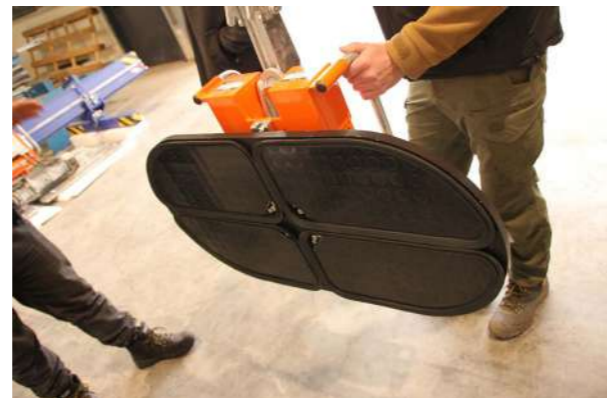
Photo 3. Required multi-section central suction cup (divided into four sections).
