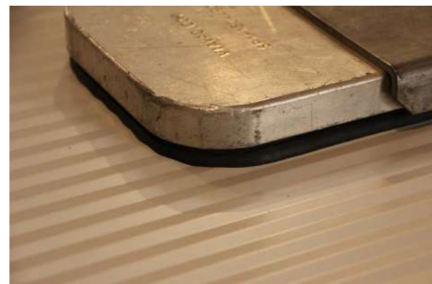
Photo 4. Low-profile suction cup for a vacuum device. Once a vacuum is created, the suction cup's flexible peripheral seal ensures support across the entire contact surface between the suction cup and the sandwich panel.
